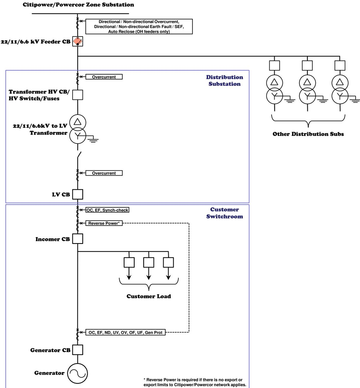
Figure 4 - Protection scheme example 2: 30kW – 200kW generation [Rotating machine].
