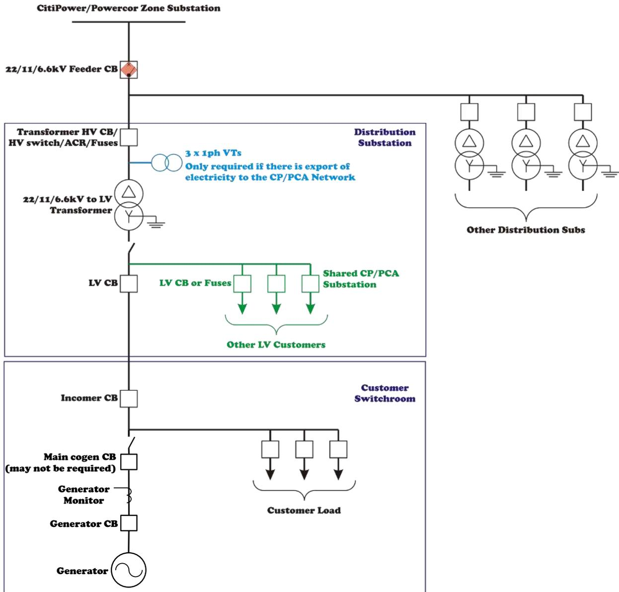
Figure 2 - LV Customer Minimum Connection Configuration
