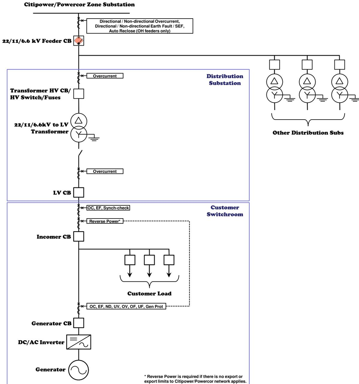
Figure 3- Protection scheme example 1: 30kW – 200kW inverter connected generation.
