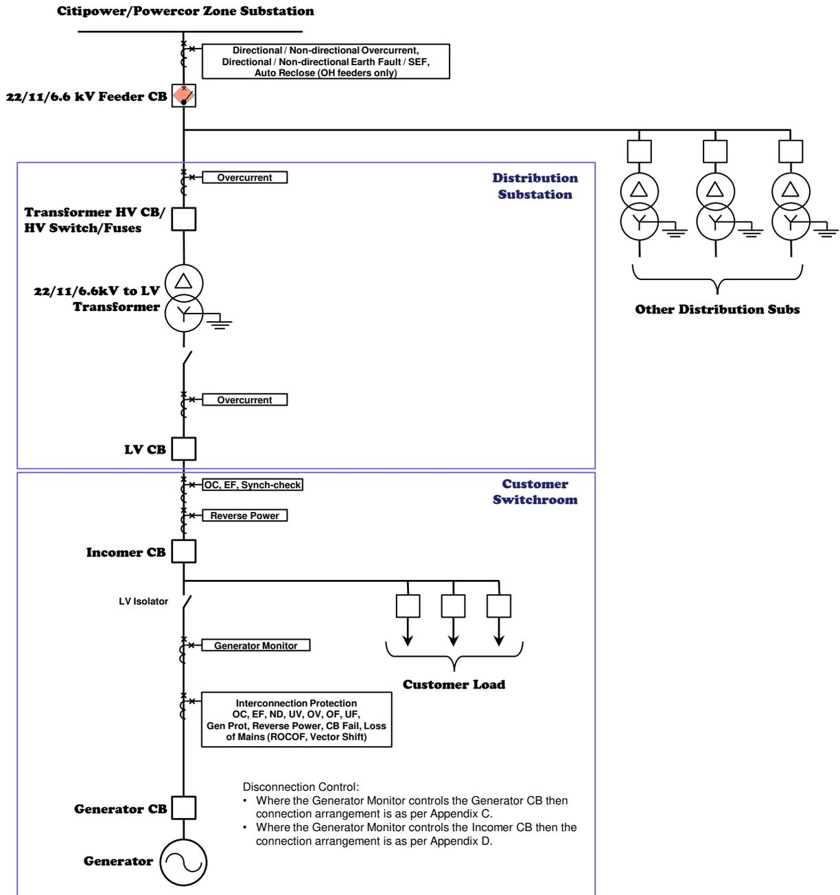
Figure 5 - Protection scheme example 3: 200 kW – 500 kW generation with export [e.g. synchronous generator].
