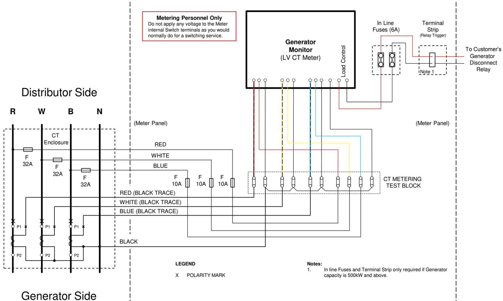
APPENDIX D – Typical Wiring Diagram for Generator Monitor (Main Co-Gen CB or Incomer CB Control)
