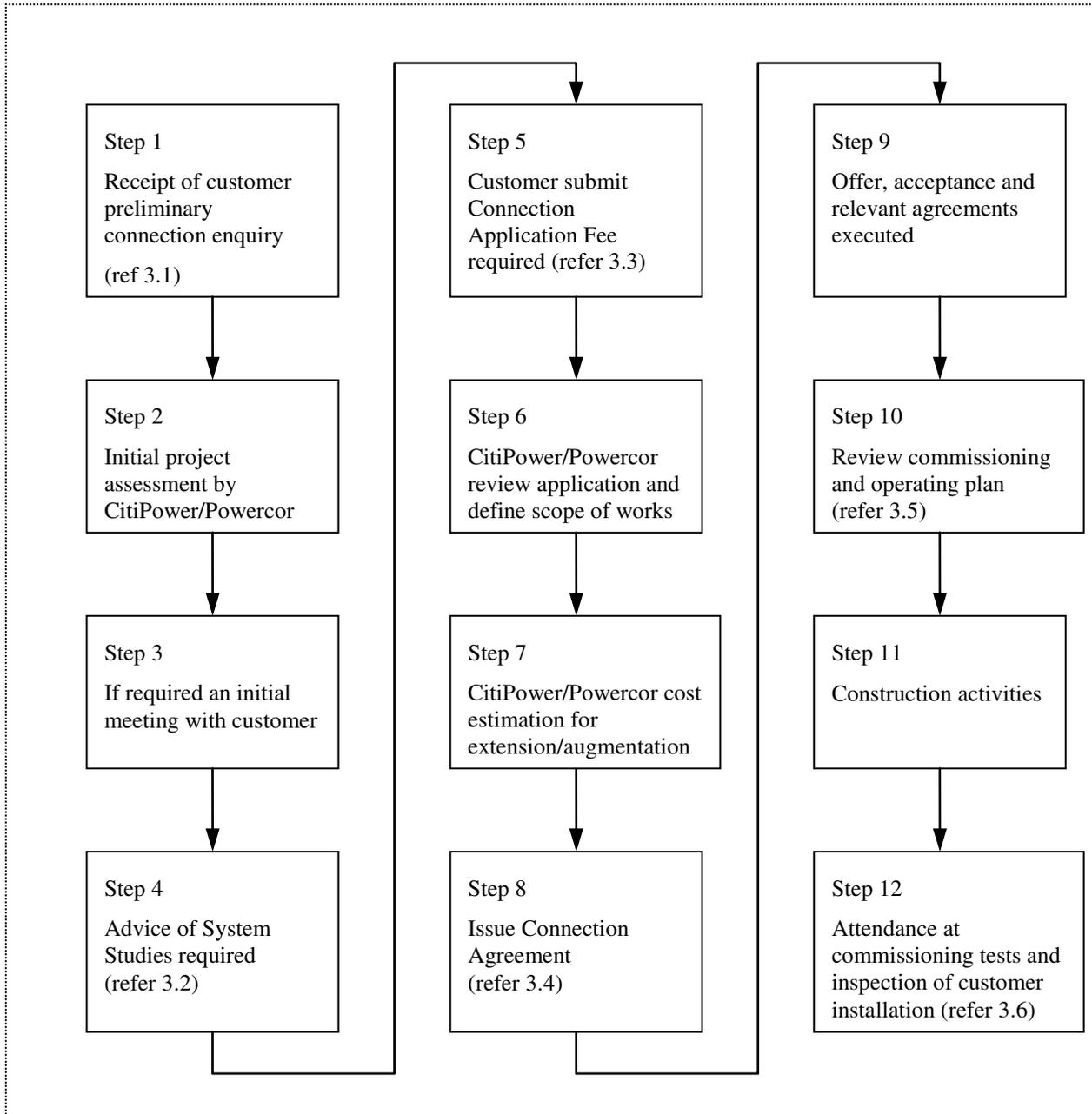
Figure 1 - Flowchart Showing LV Embedded Generation Process
